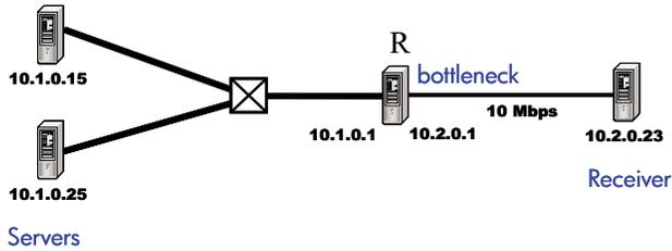
**Fig. 3.** Physical test-bed for evaluating PBE-STP implementations. All links besides the bottleneck link are 100 Mbps.
