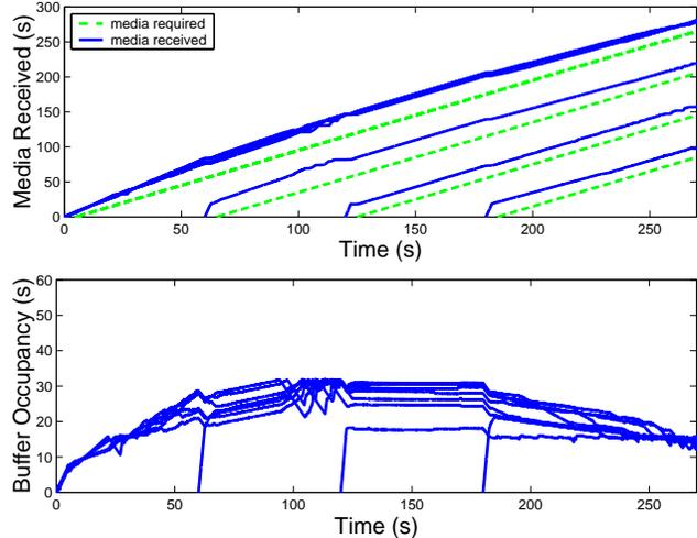
**Fig. 8.** Using hybrid priority queue, PBE-STP achieves small spread in client buffer occupancy as well as few overall number of playback disruptions.
