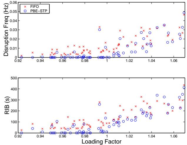
**Fig. 10.** PBE-STP achieves significantly lower Disruption Frequency and Required Initial Buffer-time (RIB) than FIFO at loading levels less than unity.
