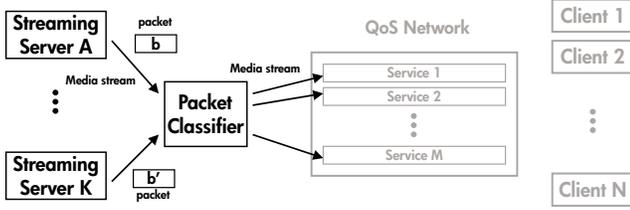
**Fig. 1.** Architecture of the proposed scheme. The network and streaming clients, which do not require modifications, are shown shaded.
