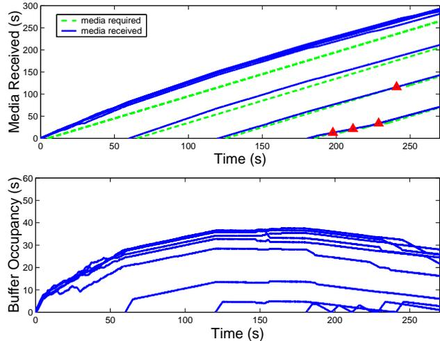
**Fig. 5.** Example illustrating the situation under conventional FIFO. Media sessions that start later (when bandwidth is constrained) have much less client buffer built up as compared to media sessions that start earlier (when bandwidth is available), and therefore are afflicted by numerous playback disruptions.
