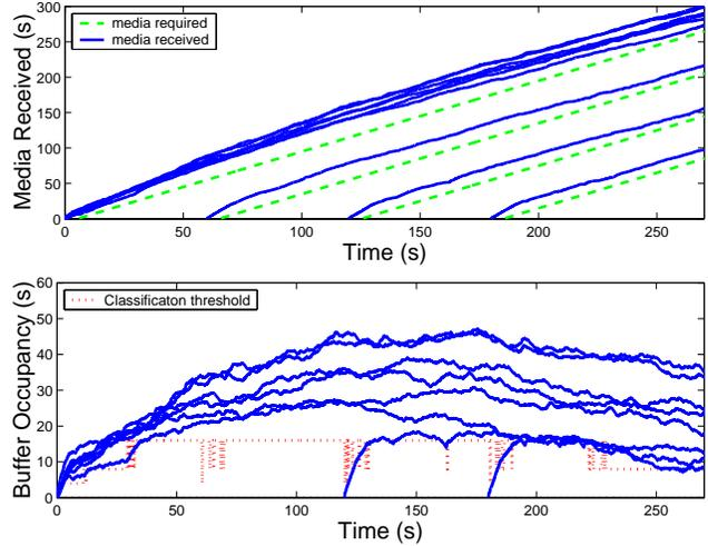
**Fig. 7.** Using a maximum of 30% premium traffic, PBE-STP reduces playback disruptions, but maintains large spread in the amount of client buffer occupancy.
