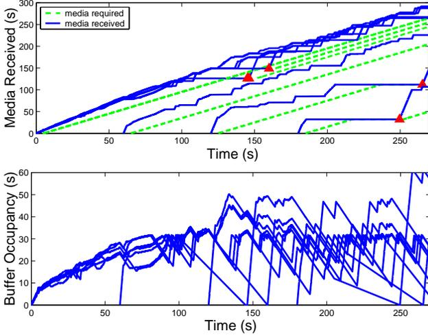
**Fig. 6.** Using priority queues, PBE-STP allows sessions starting at different times to achieve roughly the same client buffer occupancy. Nevertheless, long periods of zero throughput are observed.
