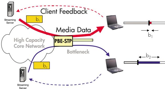
**Fig. 2.** PBE-STP exploits behaviour of congestion control mechanisms to achieve preferential allocation of resources.
