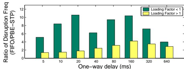
**Fig. 12.** Relative performance improvement of PBE-STP over FIFO, as a function of one-way propagation delay.
