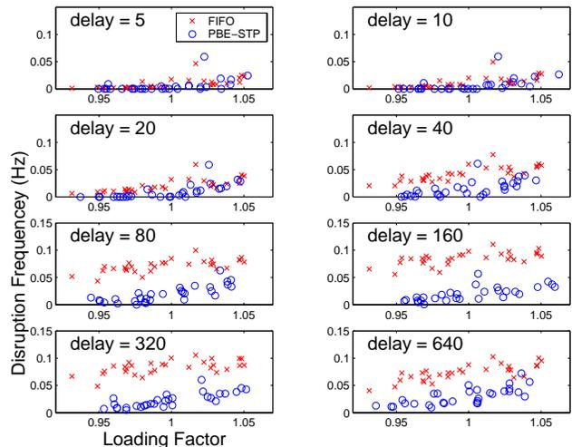
**Fig. 11.** Disruption Frequency for FIFO and PBE-STP for different one-way propagation delays.
