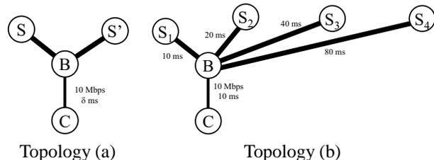
**Fig. 9.** Simulation topologies. Unless otherwise indicated, links are 100 Mbps and with negligible delay.
