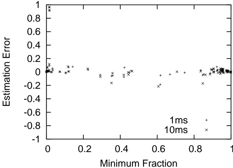
Figure 19: Scatterplot of SCONE’s estimation error with probe flows having a period of  $1ms$  and  $10ms$  sub-flows extracted from these flows.
