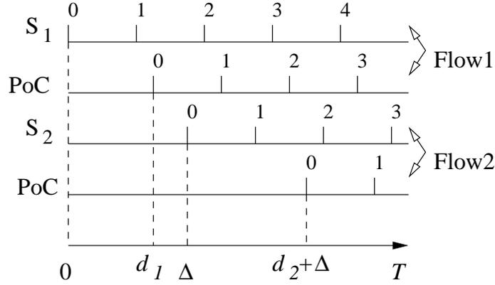
Figure 2: An illustration of synclag ( $= \Delta + d_2 - d_1$ ) of  $F_2$  with respect to  $F_1$  when the time at two sources  $S_1$  and  $S_2$  differs by  $\Delta$  and have a delay of  $d_1$  and  $d_2$  to the shared PoC. A packet sent at time  $t$  by  $S_2$  traverses shared links at around the same time as a packet sent at time  $t + \text{synclag}$  by  $S_1$ .
