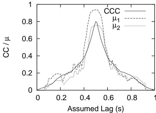
Fig. 3. An Illustration of the synclag where cross correlation and the output of CD-DJ achieve maximum
