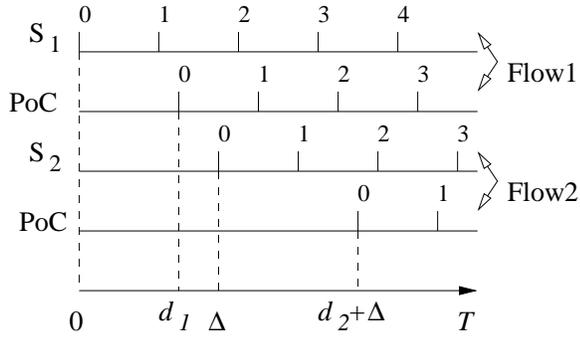
Fig. 2. An illustration of synchronization lag  $\Delta + d_2 - d_1$  when the two senders  $S_1$  and  $S_2$  start within  $\Delta$  of each other and have a delay of  $d_1$  and  $d_2$  to the shared PoC
