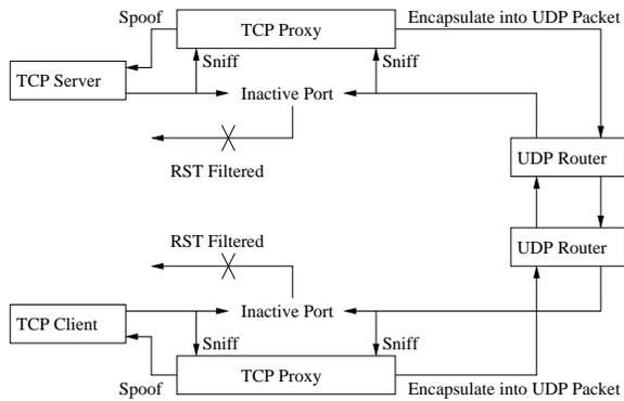
Fig. 8. An Illustration Explaining the TCP Proxy Implementation
